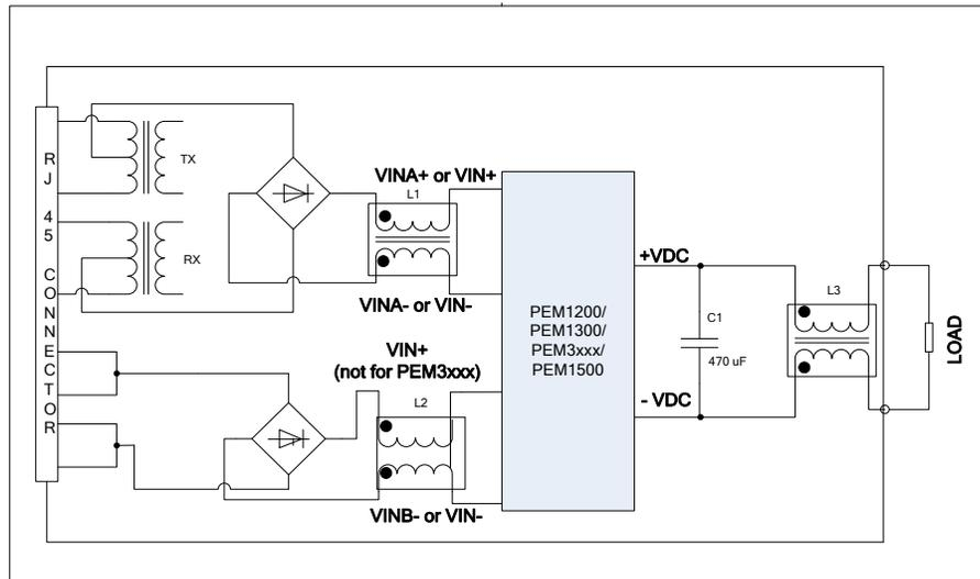
Figure 4. Common mode filters
