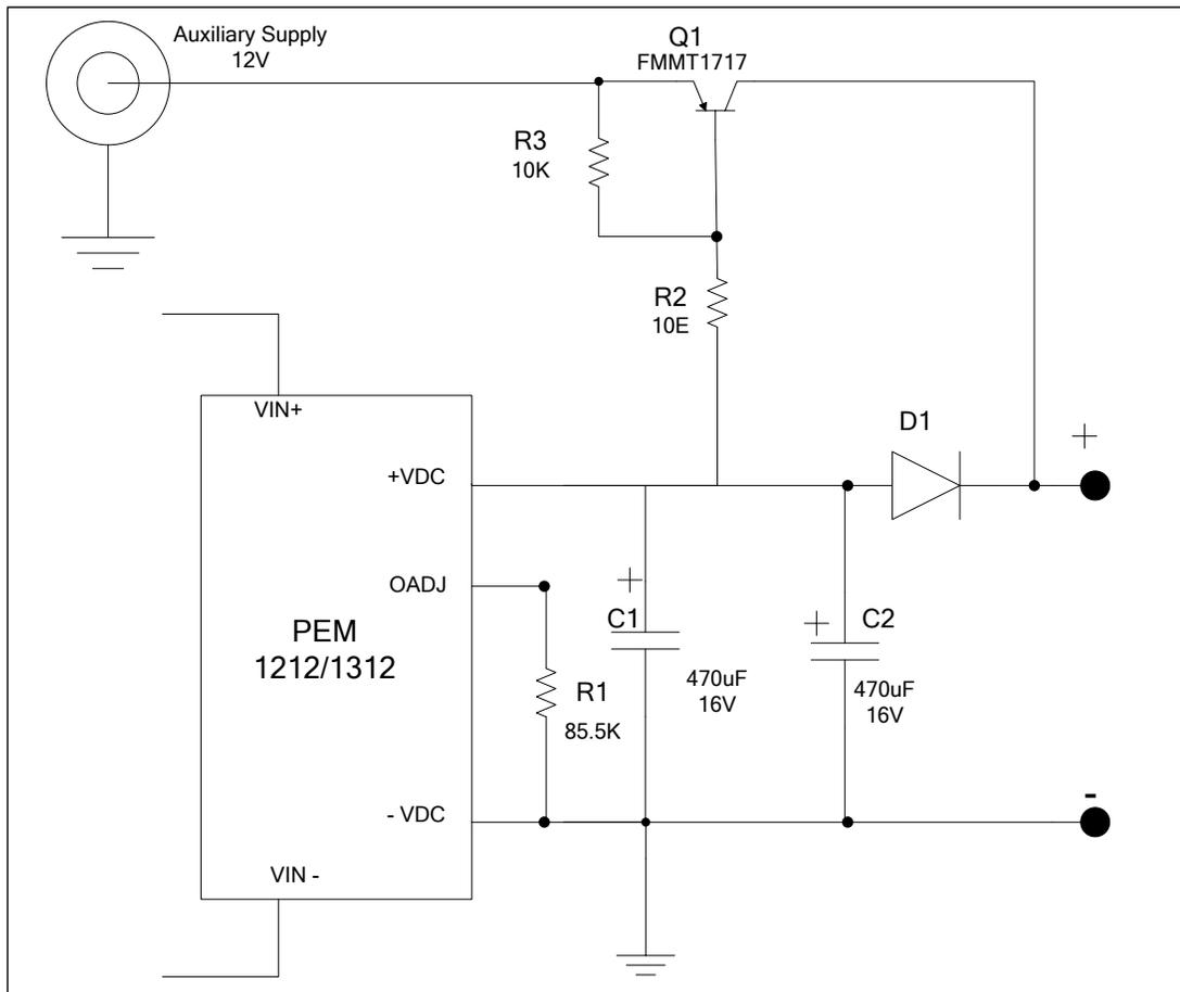
Figure 3. POE supply having priority over Auxiliary power supply.
