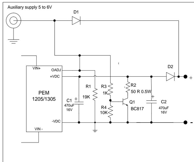
Figure 2: Auxiliary power supply having priority over POE.
