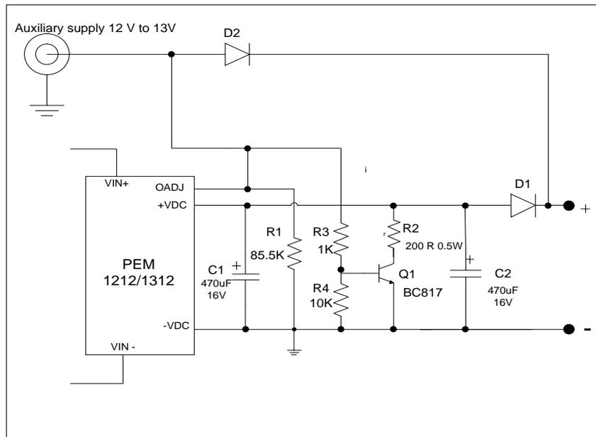
Figure 1: Auxiliary power supply having priority over POE
