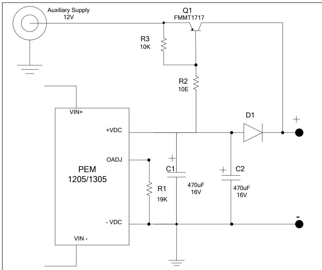
Figure 4: POE supply having priority over Auxiliary power supply.
