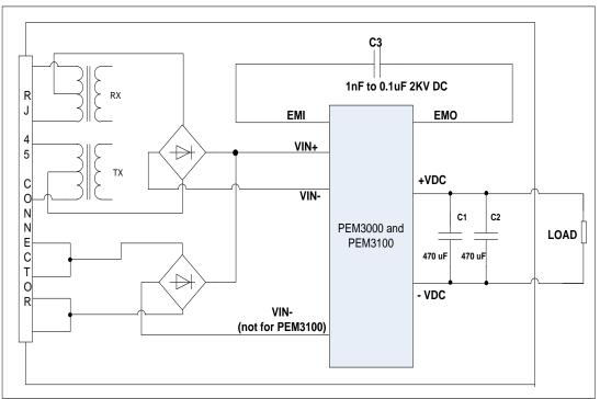
Figure 2. EMI filtration using EMI and EMO pins applicable for PEM3000 and PEM3100 series only
