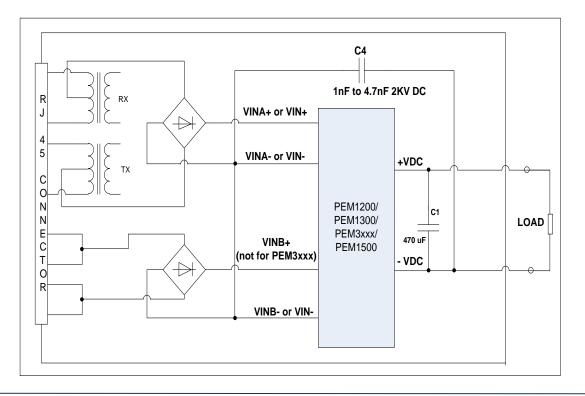
Figure 1. EMI filtration using safety capacitor
