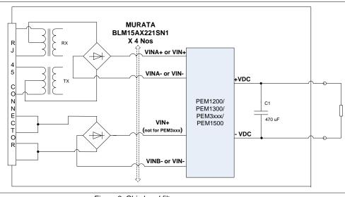
Figure 3. Chip bead filter
