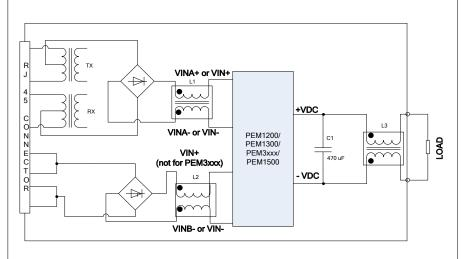
Figure 4. Common mode filters
