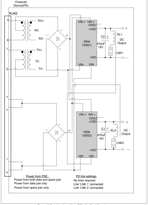
Figure.5 Combination of two PD's for Dual Supply
