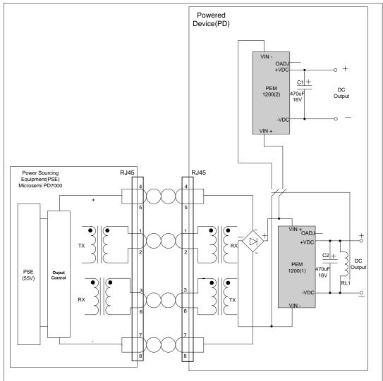
Figure.2 PD with Microsemi PSE equipment
