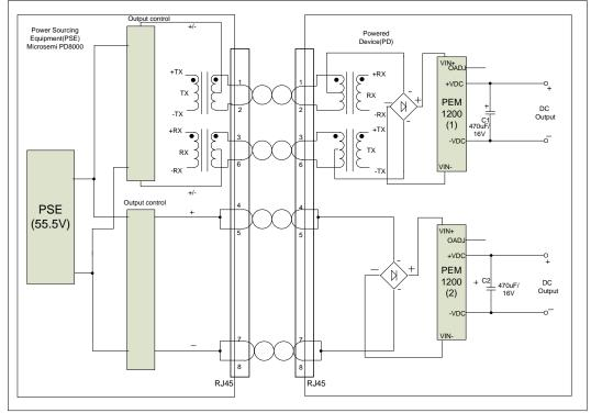
Figure.1 PD with Microsemi PSE equipment
