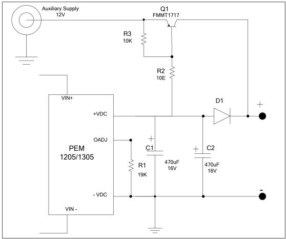
Figure 4: POE supply having priority over Auxiliary power supply. Example device used PEM 1205 and PEM1305.
