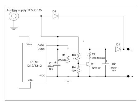
Figure 1: Auxiliary power supply having priority over POE Example device used PEM1312 or PEM1212.
