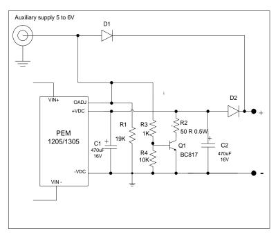
Figure 2: Auxiliary power supply having priority over POE. Example device used PEM1205 or PEM1305.
