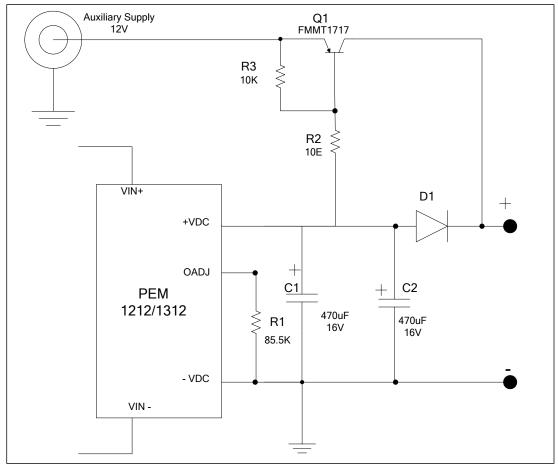
Figure 3. POE supply having priority over Auxiliary power supply. Example device used PEM 1212 and PEM1312.
